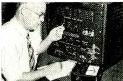
Dynamic Fluxmeter, developed by Bell Laboratories, indicates flux build-up in intervals of 25 millionths of a second. Precise information like this was essential to higher speed operation.
