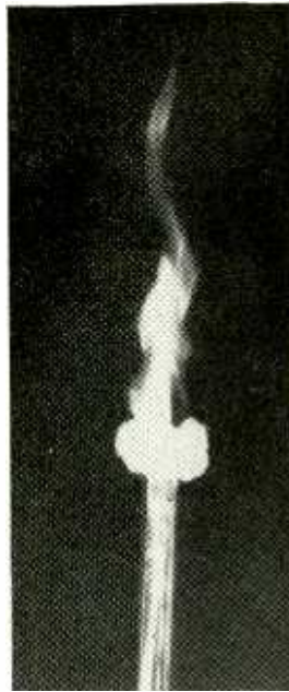
Zinc rod, showing the formation of oxide as the flame consumes it.
