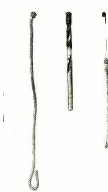
Fig. 2—Copper wire, steel drill and iron clothesline after burning. The single strand of clothesline was observed to burn down one inch in ten seconds.
